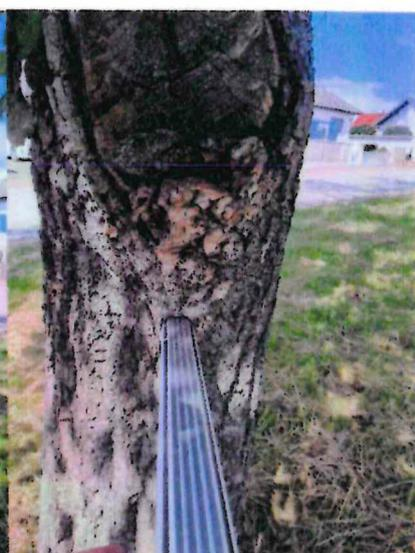
Abb. 3: Messung Resistograph
